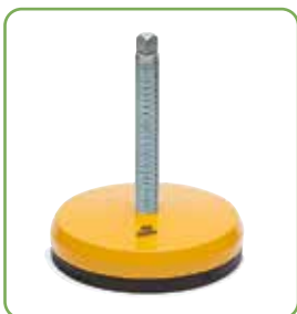
Part. R0406 - Pag. R39 Ø 123 • Painted steel • Max. load 50000 N.
