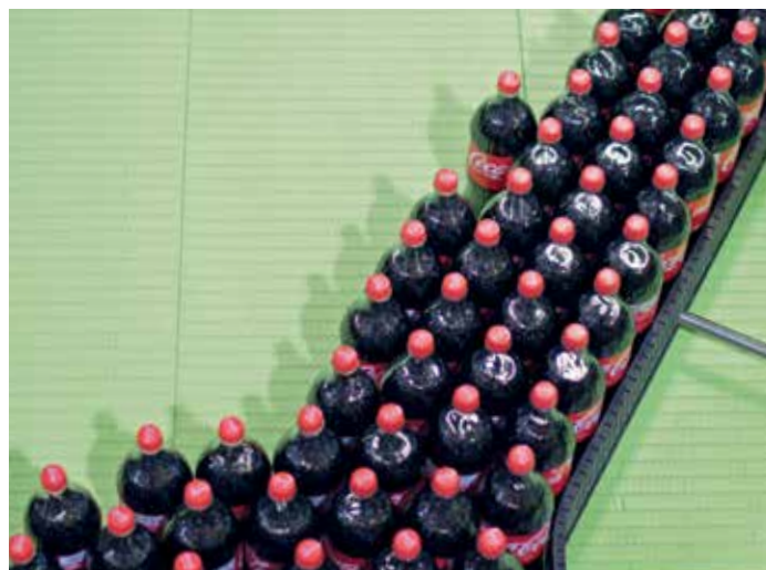
Bottle conveyor with FT1000 DRY-PT MatTop® Chain
