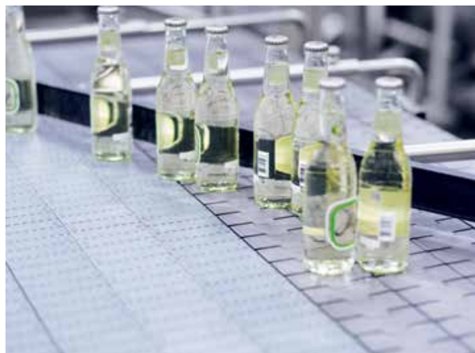
Bottle conveyor with FT1000 PSX MatTop® Chain
