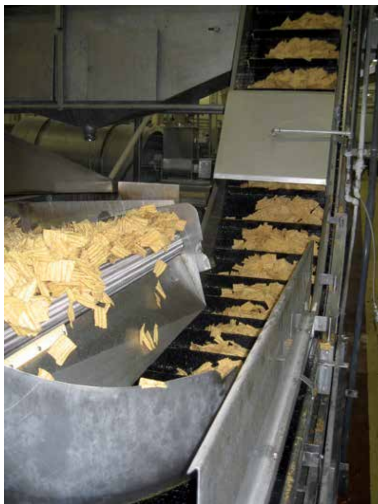
Inclined conveyor for chips FTR2015 mattop chain
