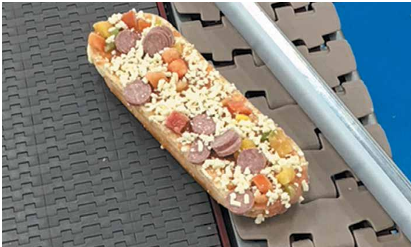
Conveyor equipped with Rexnord 395 Series KleanTop Belt.
