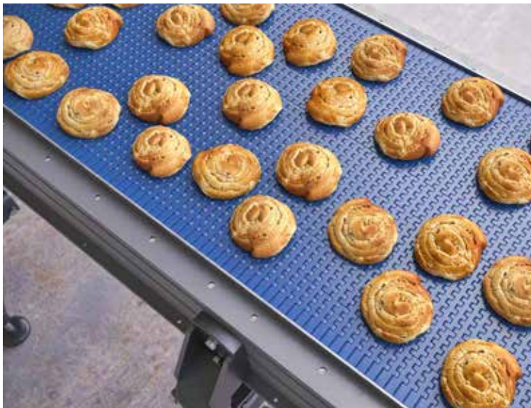
Conveyor equipped with Rexnord 595 Series KleanTop Belt.
